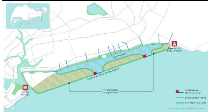
Fig 2: Planned ‘Long Island’ reclamation in East Coast
